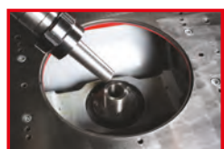
Wechselspindel MK4 exchangeable spindle MT4
