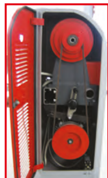
stabiler Riemenantrieb solid and smooth belt run
